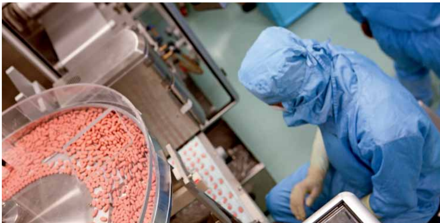
Blister Packing Line, Ranbaxy Plant, Paonta Sahib, India
