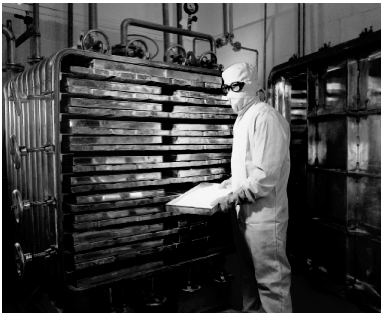
Raking Operation in Vacuum Tray Drier
