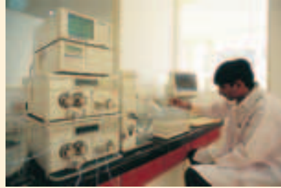
Preparative HPLCs are used for peptide purification
