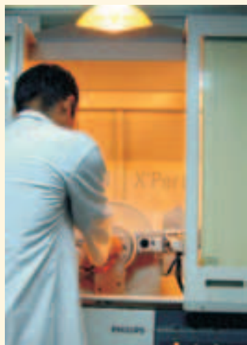
Above: USFDA approved bulk active plant, Ahmednagar Below: X ray diffractometer, analytical lab, SPARC Tandalja
